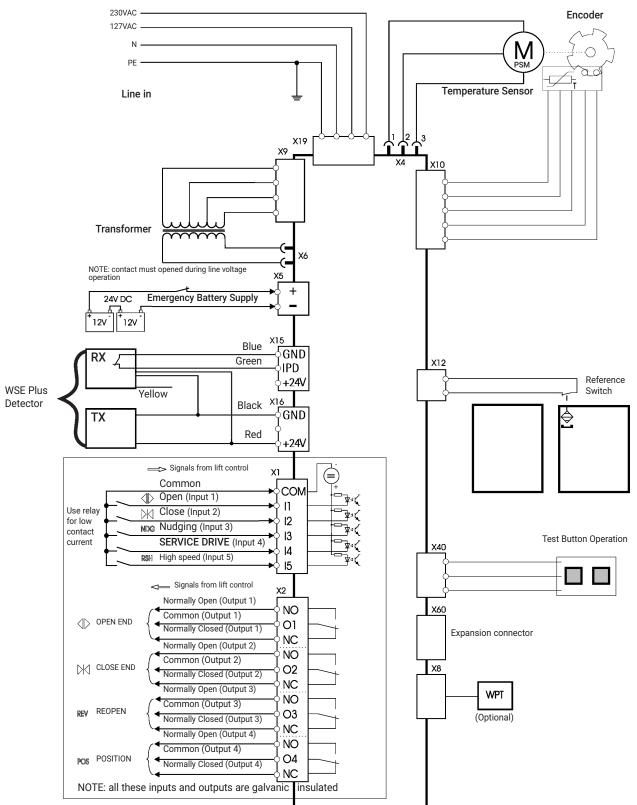
For Parameterset xE (EN81-20) the IPD input have to be always active for normal operation.
